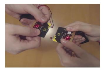
The Micro:Bits will be connected via the radio module on each of the Micro:Bits so they can communicate to each other during the game.
